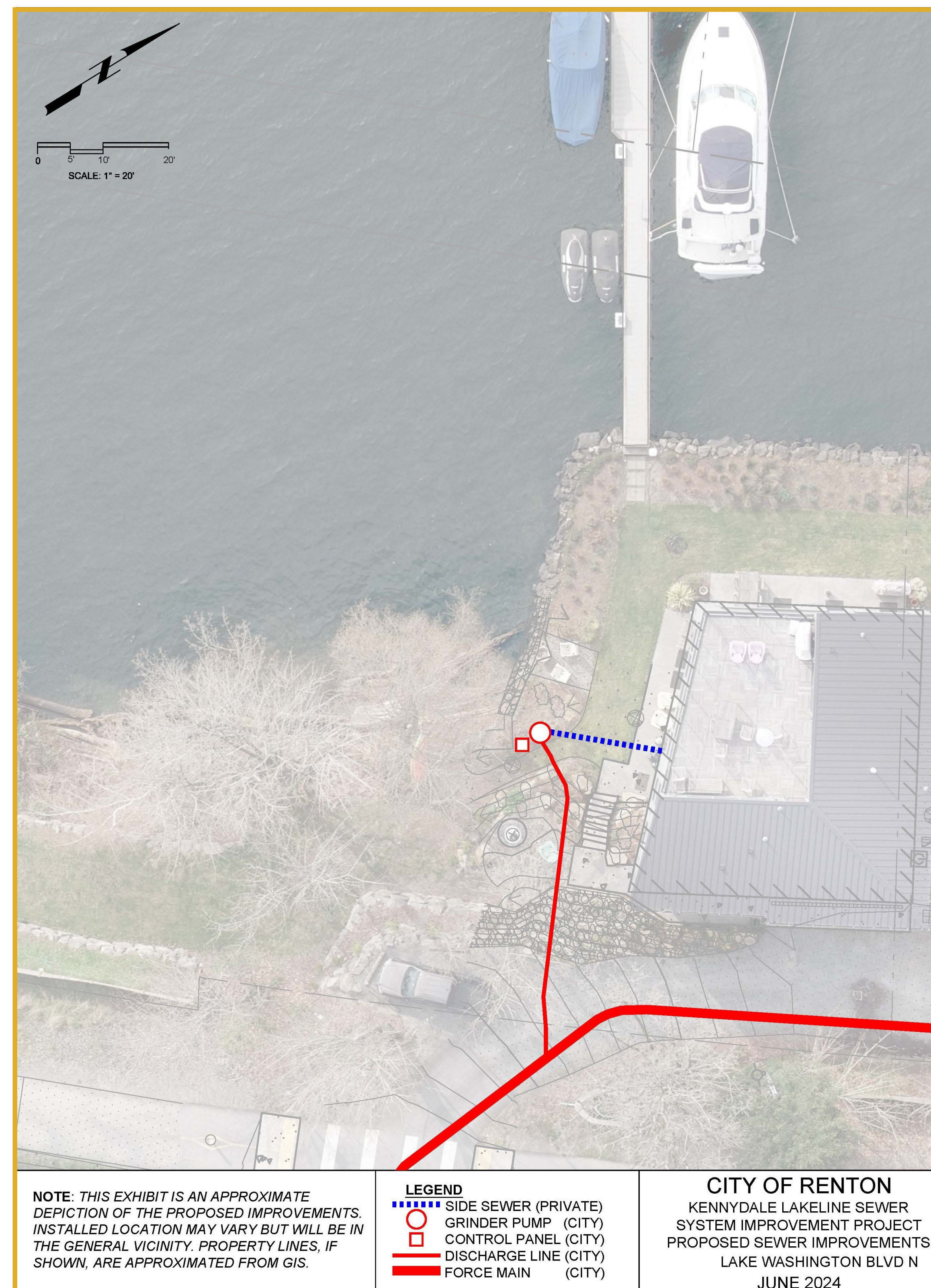
Depiction of typical land-based system elements once installed.
