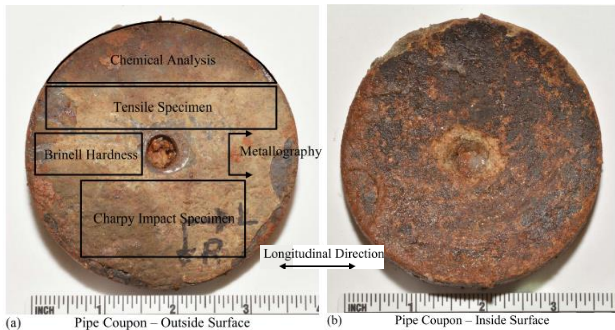
Figure 2-1. Pipe Coupon as Received by Laboratory
