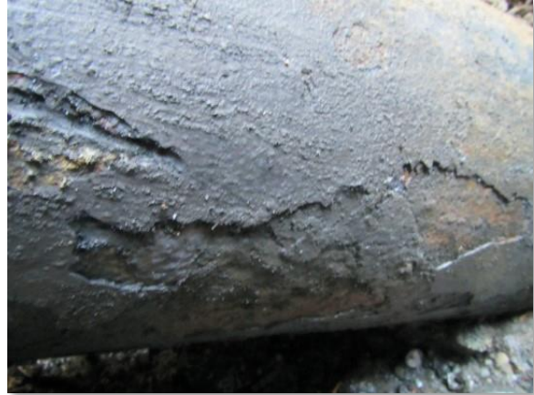
Photo C-4. Lower half of Lakeline with graphite scale
