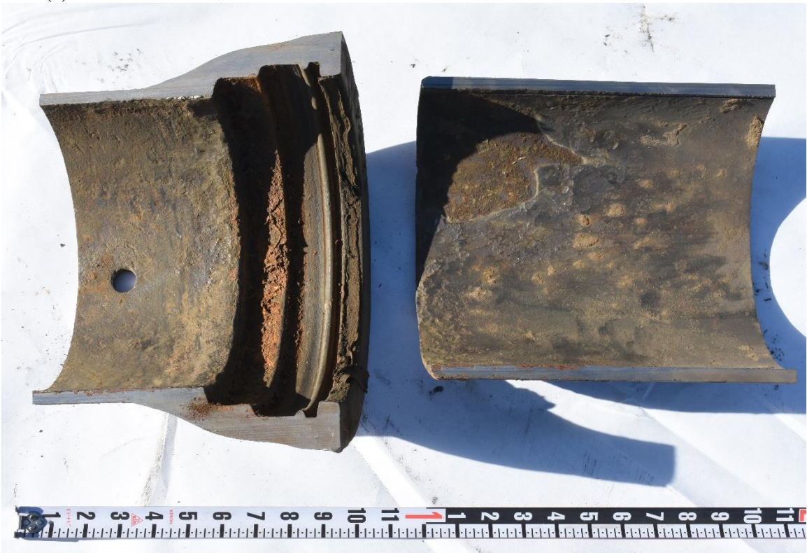
Figure 7 Photographs of the bell side of Manhole 5 after wire wheel brushing.
