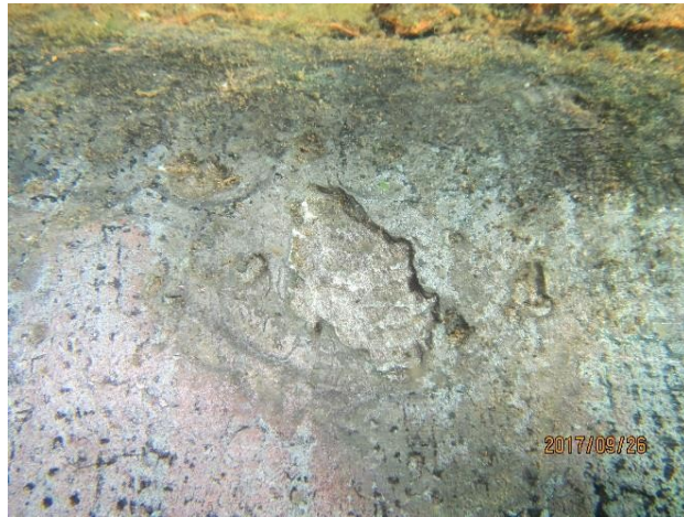
Figure 6.1-5 Pitting and Graphitization
