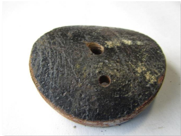
Photo 3-8. Exterior surface of lateral coupon with minor pitting corrosion.
