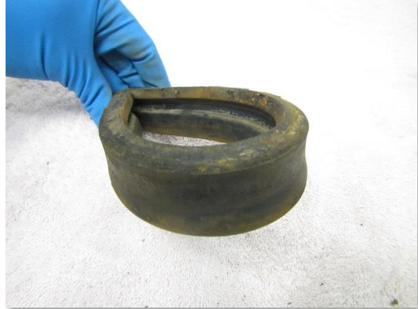
Photo 3-12. Rubber gasket was pliable and in good condition with no cracks. Photo shows the inside surface of the gasket half, bent inside-out.
