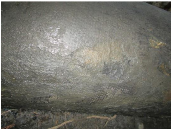
Photo C-5. Dimpled surface indicative of DIP
