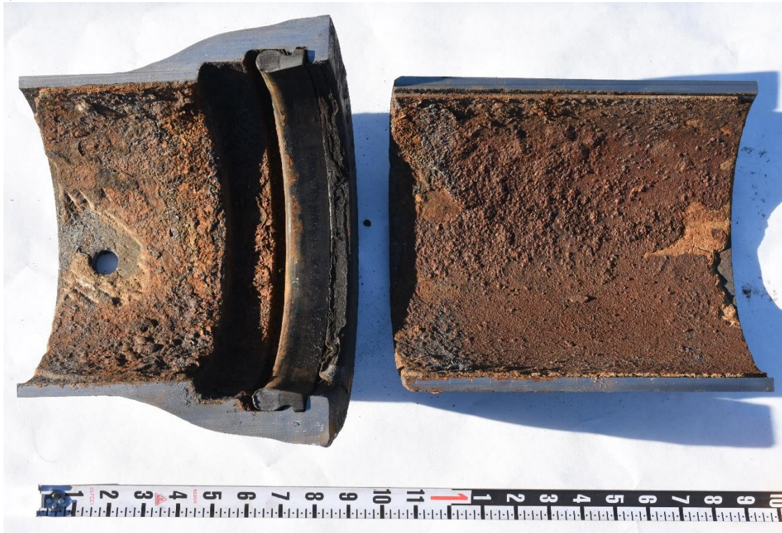
Figure 5 Photographs of the inside surfaces of the bell side of Manhole 5 after longitudinal sectioning.
