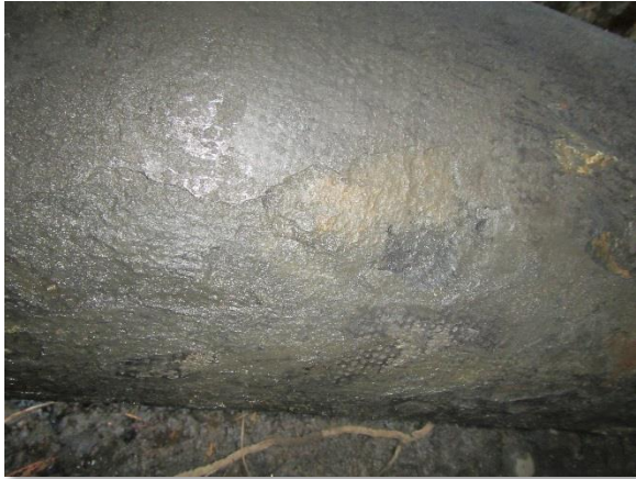
Photo 2-16. Dimple pattern (DI pipe); pitting and graphitization
