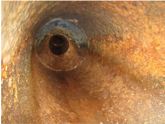
Photo 2-16. Dimple pattern (DI pipe); pitting and graphitization
