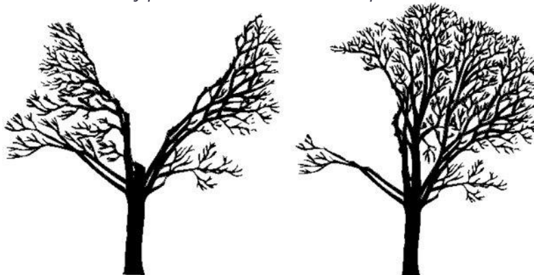
Figure 36. Example of trees directionally pruned for clearance from power lines
