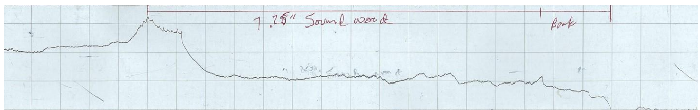
Figure 8. Resistograph tape showing the thickness of sound wood.
