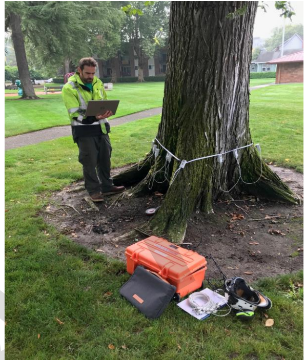
Figure 7. Tomograph measurements being taken on a tree in Jones Park, Renton, Washington.
