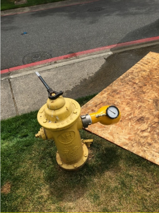
Hydrant Set-up for one of the fire flow tests
