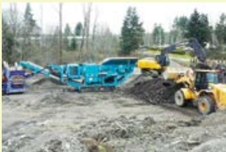
**City maintenance shops recycle and/or reuse project construction debris.** This allows for the recovery of topsoil and structural fill that can be used in other projects rather than sent to landfill. The process also saves money by reducing the amount of fill material and topsoil the city must purchase. This program saves \$50,000 to \$80,000 per year.
